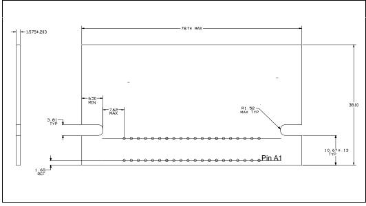
Figure 4. Voltage Regulator Module Printed Wiring Board Features (Viewed from connector side, dimensions in mm)
