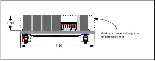
Figure 2. Module Top View (dimensions in inches)
