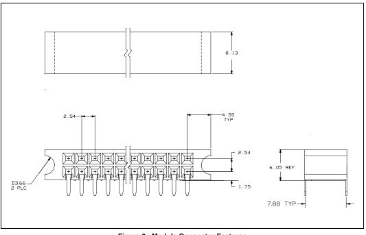
Figure 3. Module Connector Features (dimensions in mm)
