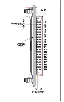
Figure 1. Pin Orientation
