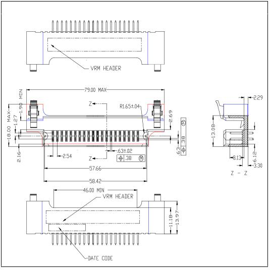
Figure 5. Mating Header (dimensions in mm)
